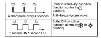
With the boiler switched ON (\*\* or \*\*) all the lamps (12 in Fig. 2) are activated.
